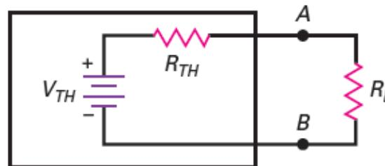
$$V_{TH} = V_{OC}$$
