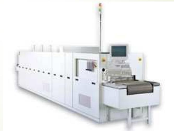
Belt speed and heater temperature sets the profile.
