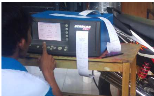
Fig.5. Data collection process during exhaust emission gas testing
